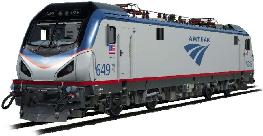
The Northeast Corridor has been home to a long lineage of famous electric locomotives, including the Pennsylvania Railroad's iconic GG1 and Amtrak's long-lived AEM-7. Today's standard-bearer on the NEC is the ACS-64 ("ACS" stands for "Amtrak Cities Sprinter"). Constructed by Siemens Mobility, a subsidiary of Siemens AG of Germany, the stylish electric locomotive's design is based on the successful EuroSprinter. Amtrak has purchased 70 ACS-64s, the first of which entered service in February 2014.
